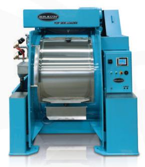
The cylinder's smooth finish helps to minimize degradation of the items processed and significantly reduces the production of lint.
